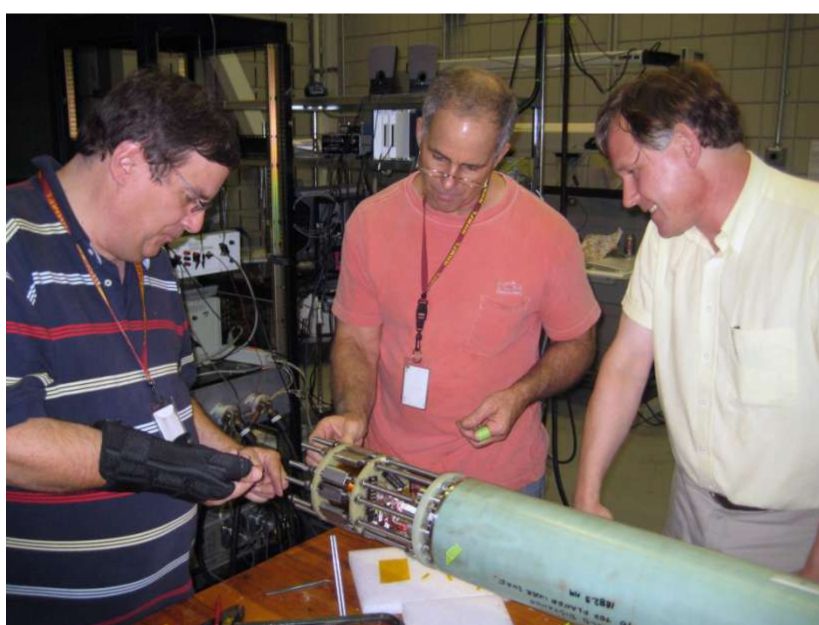
Above: Scientists building a test coil for a 32 tesla superconducting magnet
